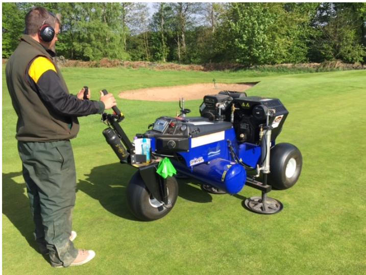
Installed at Woolley Park 12 months ago, regular use of this state of the art aerating machine has immediately improved drainage by creating larger pore space in our soil subsurface. This has enabled us to be one of the few courses open in our area on some of the wettest days the 2015/16 winter has offered up.
